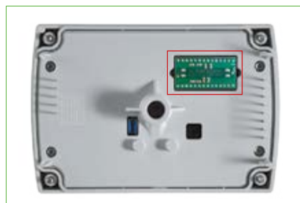
RS485 - Modbus RTU
